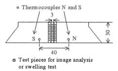
(b) Rubber sample, Cross section A-A
