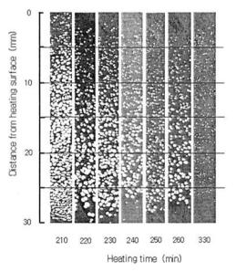
Fig. 3. Binarized images of cell structure for  $\tau_{H}$  = 210~330 min.
